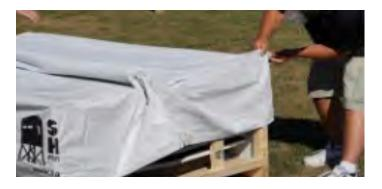
Disassemble shipping container by pulling off Tyvek wrap and removing screws from the protective wood top. Cut plastic bands and remove.
