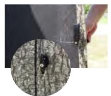
Insert the outside door handle through the pre-drilled hole in the door.
